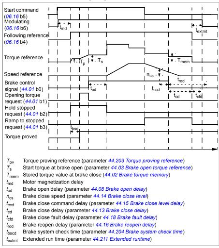
**Note**: In case of any fault, the brake closes immediately. By default, the brake control uses relay output RO1.
