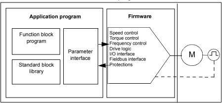
The firmware program performs the main control functions, including speed, torque and frequency control, drive logic (start/stop), I/O, feedback, communication and protection functions. Firmware functions are configured and programmed with parameters, and can be extended by application programming
