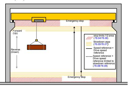
The crane slowdown function uses Limit to limit trigger type Level low (76.03) and has two modes:
