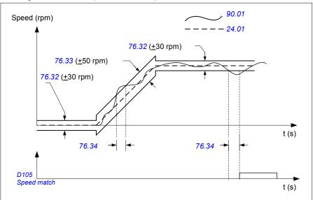
The diagram shows the operation of the Brake slip at standstill2 warning.
