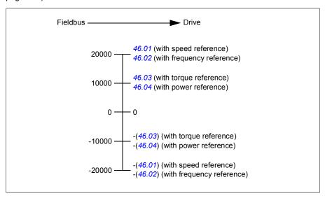
The scaled references are shown by parameters 03.09 EFB reference 1 and 03.10 EFB reference 2.
