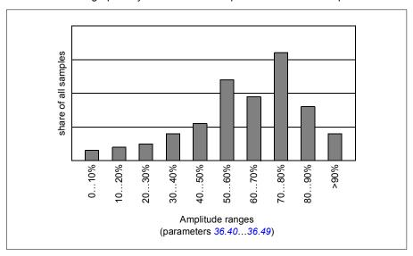
Amplitude logger 1 is fixed to monitor motor current, and cannot be reset. With amplitude logger 1, 100% corresponds to the maximum output current of the drive ( $I_{max}$ ). The maximum output current values are listed in the section *Ratings* in the *Hardware manual* of the drive. The measured current is logged continuously. The distribution of samples is shown by parameters 36.20...36.29.
