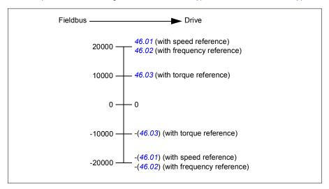
The scaled references are shown by parameters 03.05 FB A reference 1 and 03.06 FB A reference 2.
