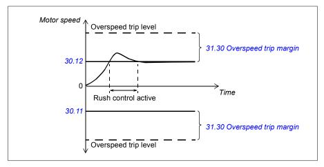
The function is based on a PI controller. The program sets the proportional gain to 10.0 and integration time to 2.0 s.
