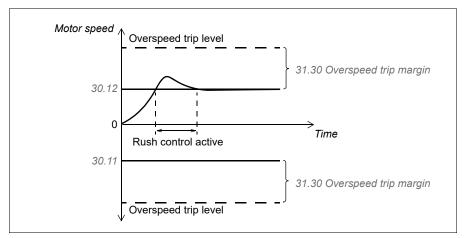
The function is based on a PI controller. The program sets the proportional gain to 5.0 and integration time to 2.5 s.
