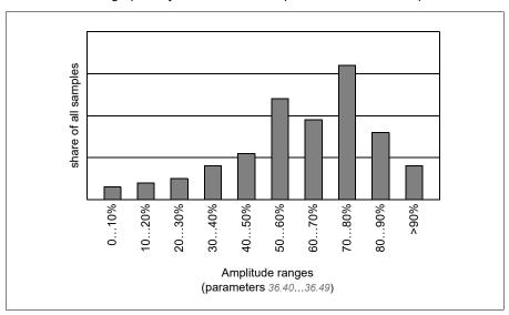
Amplitude logger 1 is fixed to monitor motor current, and cannot be reset. With amplitude logger 1, 100% corresponds to the maximum output current of the drive  $(I_{\text{max}})$ . The maximum output current values are listed in the section *Ratings* in the Hardware manual of the drive. The measured current is logged continuously. The distribution of samples is shown by parameters 36.20...36.29.
