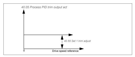
**Note:** In the above graph, it is assumed that the PID output is limited or stable at 100. This is for clarity only. In real life scenarios, the PID output can vary based on the setpoint and the actual value.
