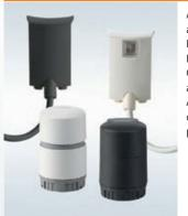
Actuators and cables are available in white or black. Positioning signals range from DC 0...10 V modulating via ON/OFF to PDM<sup>1)</sup>. Models are available for NO<sup>2)</sup> and NC<sup>3)</sup>. Actuators and cables can be ordered individually or as pre-defined product packages.
