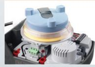
Universal accessories for easy implementation of function extensions: Whether auxiliary switch or potentiometer – all auxiliary modules can be fitted to all new types of actuators for large- and short-stroke valves. The guide rails allow easy and exact positioning of the modules.
