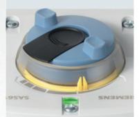
For temporary manual operation, for example during installation, just press and turn the manual adjuster, driving the actuator to the required position. When the manual adjuster is released, the actuator returns to automatic operation. The slide switch lets you fix the actuator in the desired position as long as necessary.
