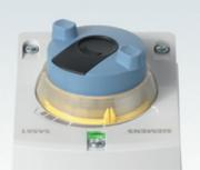
Time-saving commissioning and plant checks: Due to the well-designed position indication around the manual adjuster, the valve's travel is easy to see, even from a distance. The integral LED clearly indicates the operating status. The manual adjuster moves when the actuator operates in control mode, enabling you to check whether all large- and short-stroke actuators are working properly.
