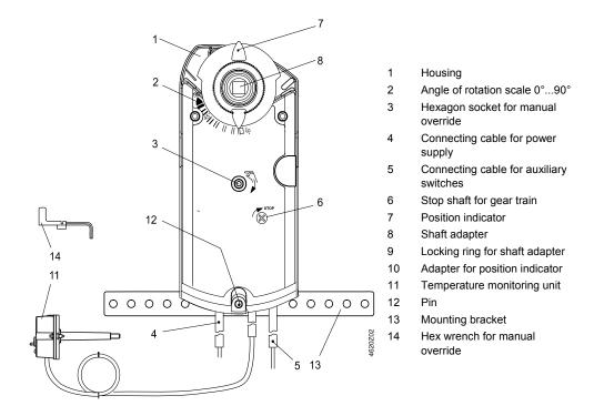
Arrangement for shaft adapters
