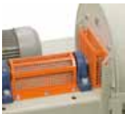
Axis protection guards and transmission in accordance with standards
