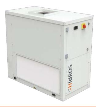
Series SDA dehumidifier are expressly designed for use in swimming pools where humidity should be closely controlled in order to guarantee optimal comfort. These units are intended to be installed in a technical room close to the swimming pool. A centrifugal fan with high available static pressure allows unit connection to ductworks, both for air suction and discharge. This series comprises 5 basic models which cover a capacity range from 73 to 240 I/24h.
